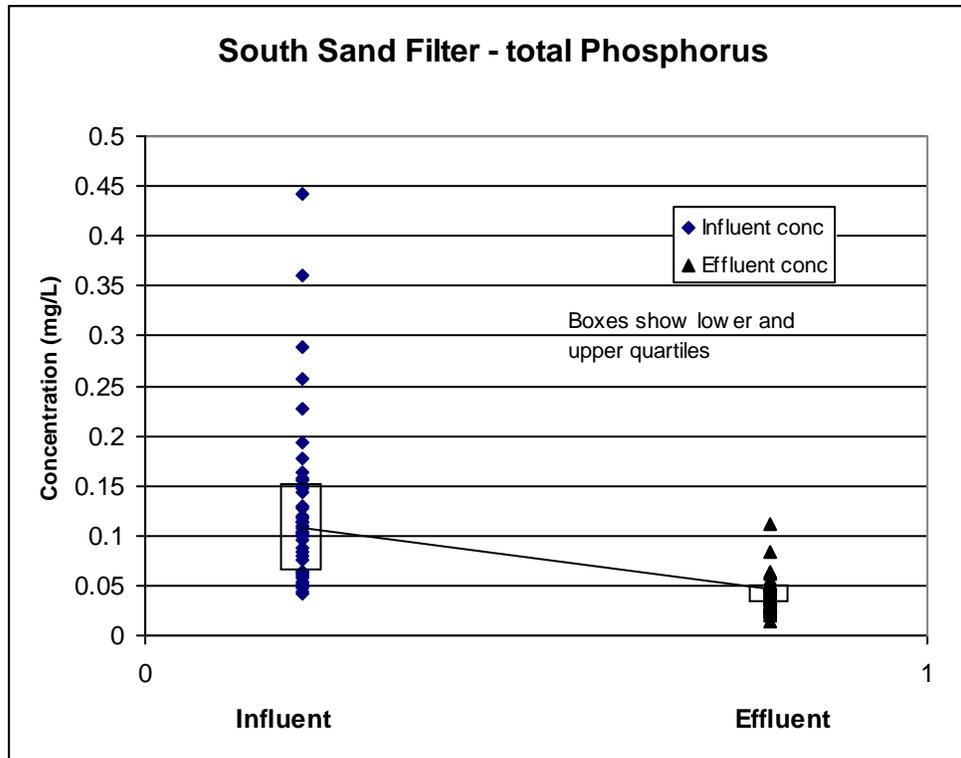
**Scatter plot: Lakemont South sand filter, phosphorus removal.**
