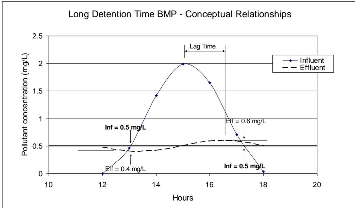
**Figure 1 - Conceptual Relationships of Influent and Effluent for BMPs with Long Detention Times**
