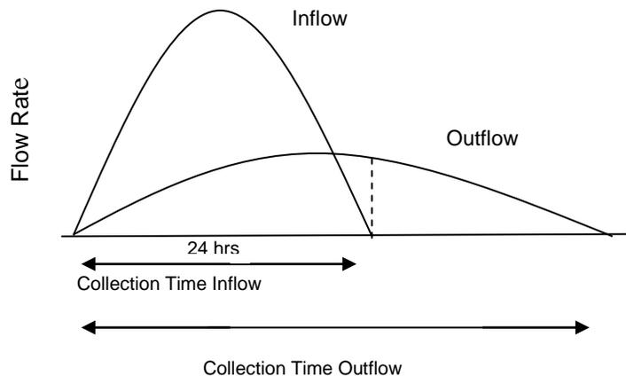
**Figure 2 - Depiction of Portions of Influent and Effluent Hydrographs for a BMP with a Long Detention Time**
