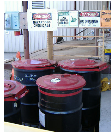
Drums on a containment pallet in a covered outdoor area
