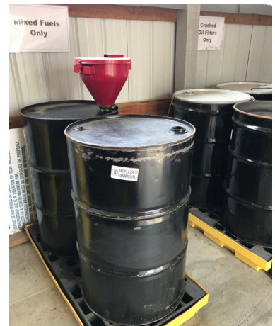
Drums on a containment pallet in an indoor area
