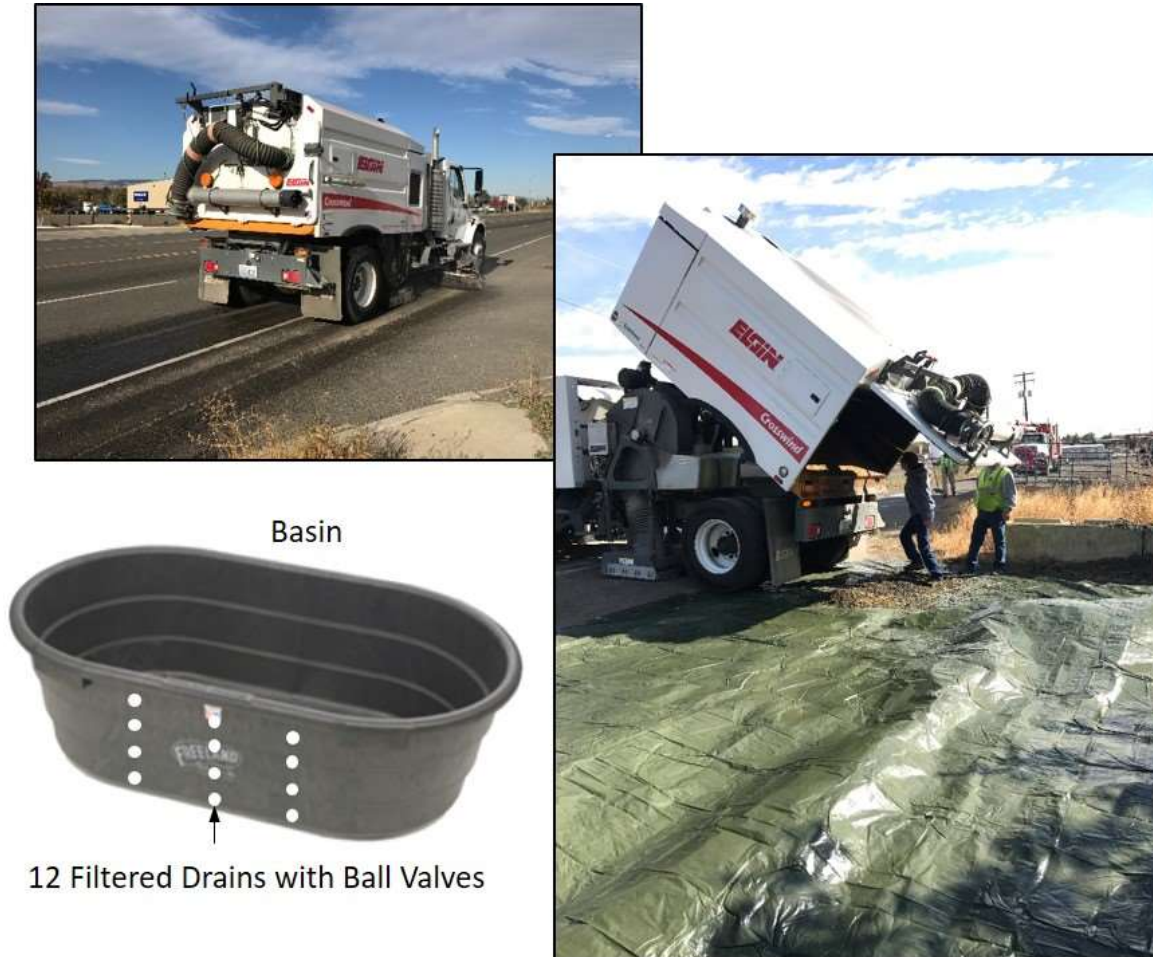
Figure 7.7 Roadway Sediment Accumulation Data Collection
