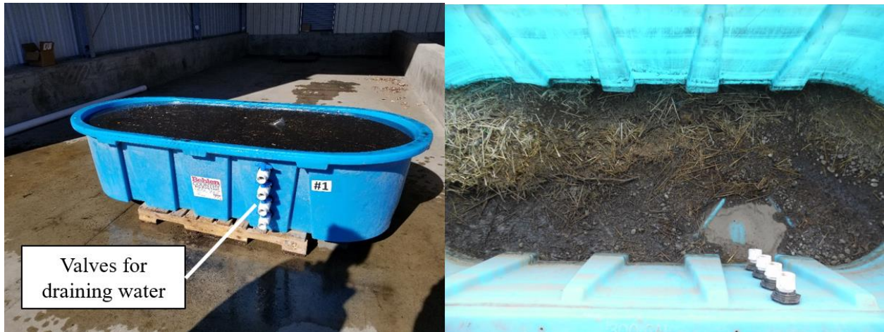
Figure 5.4 Dewatering Basin Prior to Settling (Left) and Following Dewatering (Right)
