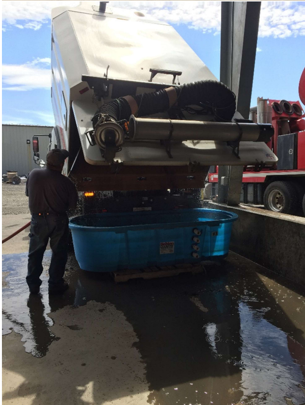
First photo shows the decant facility and basins with sweeper truck on the left and vactor truck on the right. Second photo shows the sweeper operator spraying out the inside of the debris tank to remove any remaining sediment inside the tank.
