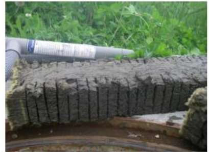
Ribbed BioMediaGREEN blocks coated with fines
