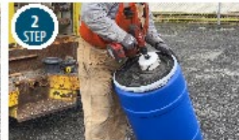
2 STEP Drill a hole in the barrel's lid. Make sure it is offset so it doesn't flow directly into the interior pipes.
