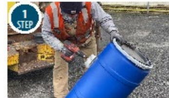
1 STEP Drill a 5-inch hole in barrel in the side of the barrel for a drain. Approximately 18 inches from the top of the barrel.
