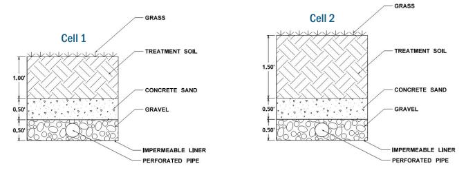
Figure 1. Cross Section of the Bioretention Cells: 12-inch BSM (cell 1) and 18-inch BSM (cell 2)
