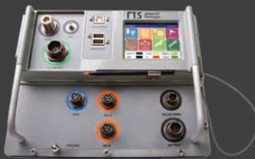
H1-RS: Rain counter, 2 SDI-12 ports, Integrated solar charge regulator
