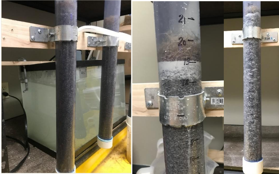
Figure 3.2 Column Testing Setup (left), Expected TSS Accumulation in Sand Filter Media (middle), and TSS Accumulation in the Sand Filter Sidewalk Vault Media (right)
