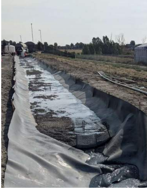
Figure D 9-14: Flow leaving swale during simulated water quality event for Alternative 4 (Photo credit: Evergreen StormH2O)
