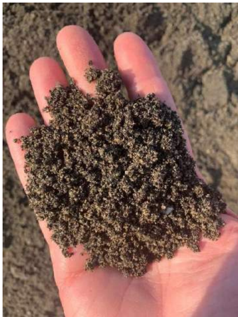
Figure D 9-13: Sample of sand media used in Alternative 4 (Photo credit: Drew Woodruff, City of West Richland)
