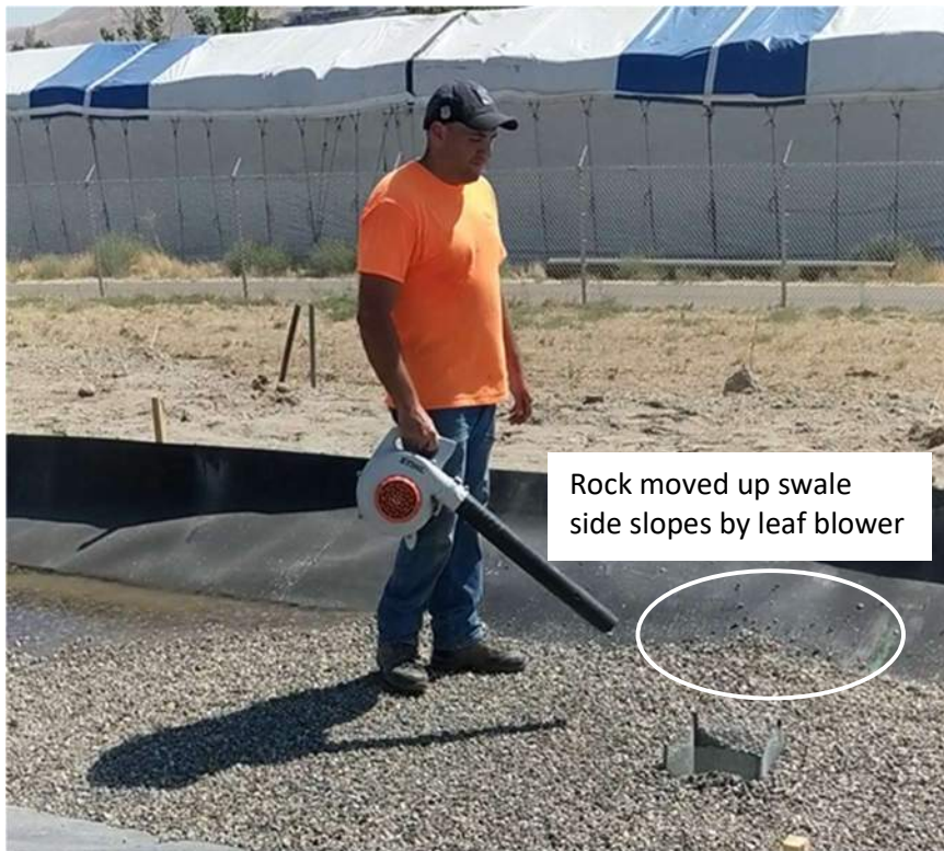
Figure D 9-5: HMA gravel movement during blower test (Photo credit: Evergreen StormH2O)
