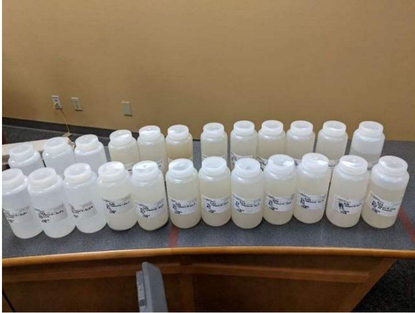
Figure D 9-2: Example of sample tint (Photo credit: Evergreen StormH2O)
